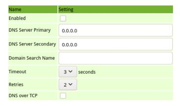
**Enabled** This setting will activate or deactivate DNS function in ROQSTAR device.
