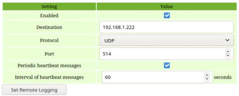
**Enable** Activate or deactivate the remote logging functionality.
