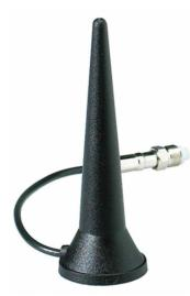
The Antenna-Magnet-L is a LTE (Long Term Evolution) antenna, which is the latest standard in mobile networking technology, referred to as 3G/4G. It covers the LTE frequency ranges of 790-960/1710-2700 MHz providing omnidirectional radiation with a gain of 2.7 dBi.
